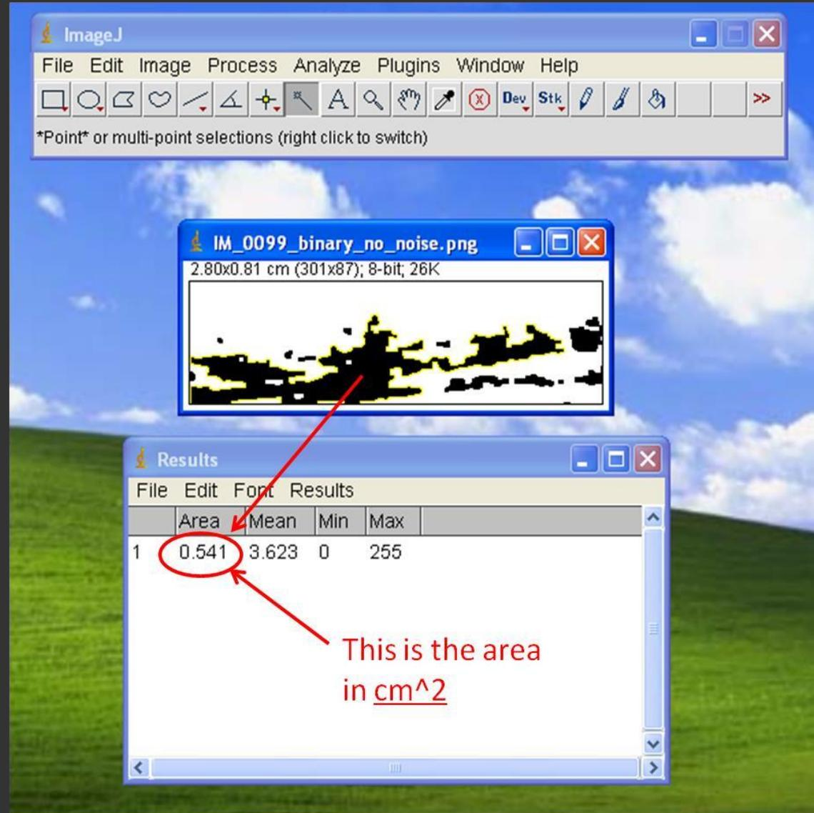
The screenshot displays the ImageJ interface. The main window shows a binary image titled "IM\_0099\_binary\_no\_noise.png" with dimensions 2.80x0.81 cm (301x87) and 8-bit, 26K. A red arrow points from the image to the "Results" window. The "Results" window contains a table with the following data:
